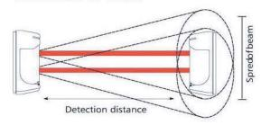
The protection distance(between Transmitter /Receiver)should be placed in the rated range.
